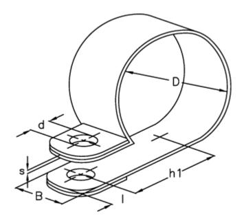
$\begin{array}{ll} d & = 4.3 \\ \text{Diameter D} = 10 \\ \text{h1} & = 9.7 \\ \text{I} & = 3.8 \\ \text{s} & = 0.4 \\ \text{Width B} & = 9 \\ \end{array}$
